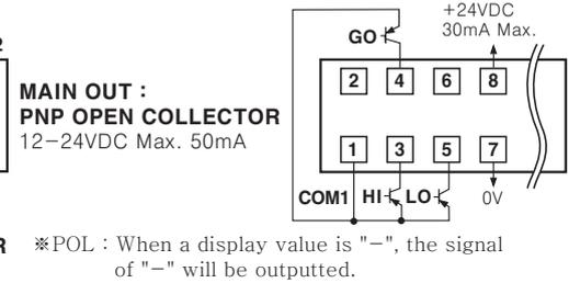
●MT4W-□□-44/ MT4W-□□-45 (Triple NPN/PNP open collector output+Transmission output)
