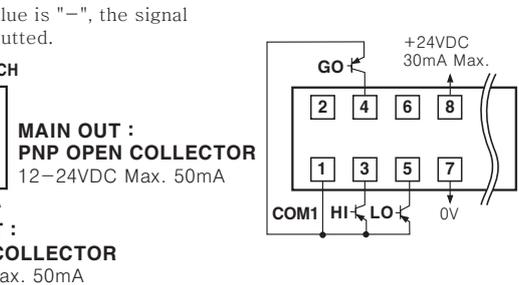
●MT4W-□□-48/ MT4W-□□-49 (Triple NPN/PNP open collector output+RS485 output)
