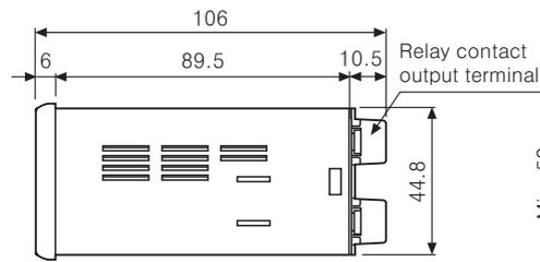
※ There is no Relay contact output terminal block in indication type.
