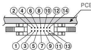
※ Hirose connector pin header model of the unit : HIF3BA-14PA-2.54DS
