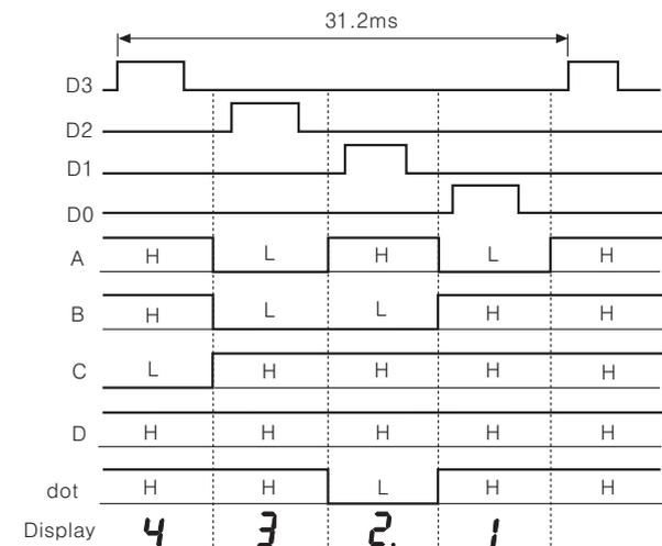
● Low speed serial output (Negative logic)
