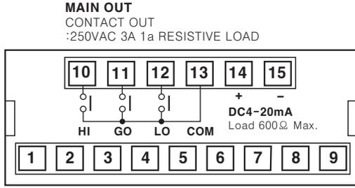
●MT4W-□□-41 (Triple relay contact output)
