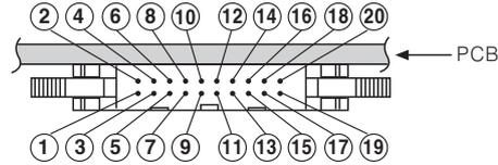
\*Hirose connector pin header model of the unit : HIF3BA-20PA-2.54DS
