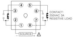
24-240VAC 50/60Hz 3.3VA 24-240VDC 1.5W
