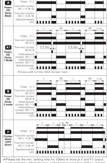
mode operation. When the min. setting time is less than 100ms, it might not be operating normally due to relay contact reaction time
