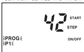
Press **MODE** key for 3sec in RUN mode, "PROG P1" is flashed.
