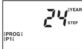
Press **MODE** key for 3sec in RUN mode, "PROG P1" is flashed and press **MODE** key 3 times more until "PROG P2 YEAR" is flashed and press **SET** key.
