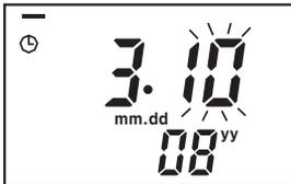
Press **▲** or **▼** keys to set 08 (year 2008) and move the flashing digit to position month by **▶** key.
