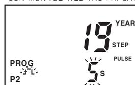
Press **▲** key 4 times to select pulse width as 5s and press **SET** key.
