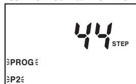
**[MODE]** key is pressed for 3sec in RUN mode, "PROG P1" is flashed and press **[MODE]** key again, "PROG P2" is flashed and press **[SET]** key.
