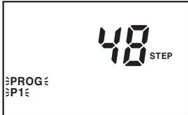
**[MODE]** key is pressed over 3sec in RUN mode, "PROG P1" is flashed and press **[SET]** key.
